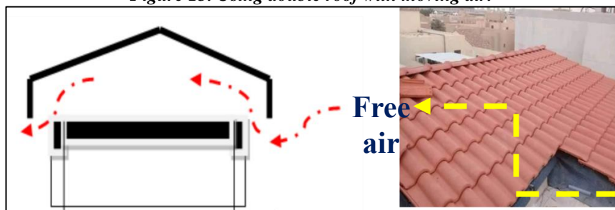
Figure 13. Using double roof with moving air.
